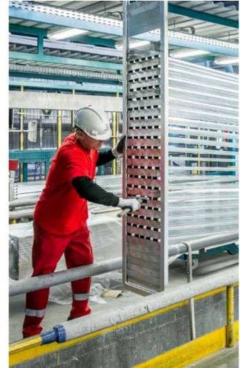
higher surface quality and colourfulness. To meet these requirements aluminium profiles are surface-treated by anodizing technology.
