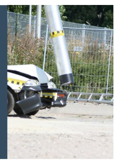
Non energy (NE) absorbing poles allow the vehicle to continue after an impact with a limited reduction in speed. They therefore represent a lower primary injury risk than energy absorbing support structures.
