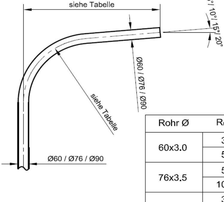
Diagram of a fixed bracket (Feste Ausleger) showing a curved pipe segment with dimensions and angles. The pipe has an outer diameter of Ø60 / Ø76 / Ø90. The bracket is labeled "siehe Tabelle" (see table) for dimensions and angles. The bracket is shown at an angle of 5°, 10°, 15°, and 20°.
