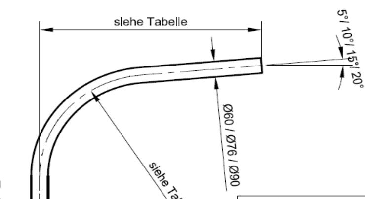
Diagram of a bracket with an invisible connection piece (Ausleger mit unsichtbarem Verbindungsstück) showing a curved pipe segment with dimensions and angles. The pipe has an outer diameter of Ø60 / Ø76 / Ø90. The bracket is labeled "siehe Tabelle" (see table) for dimensions and angles. The bracket is shown at an angle of 5°, 10°, 15°, and 20°.
